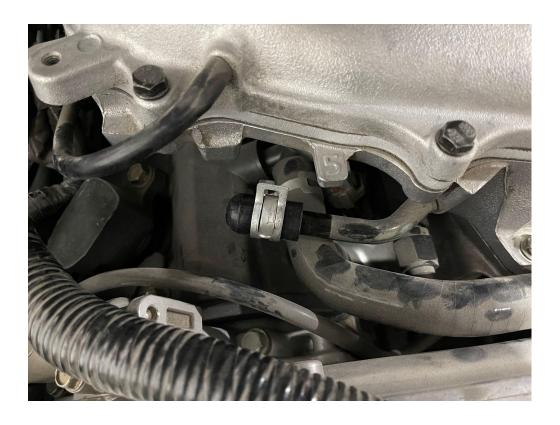
3. Remove the OEM PCV Valve using a 23mm deep well socket.
