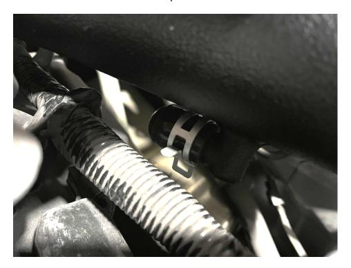
9. Install the 5/8 Vibrant filter directly to the open port on the back of the driver side valve cover and tighten the clamp securing everything in place.
