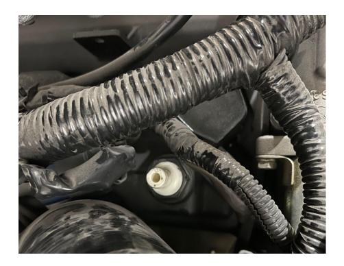
4. Install the VQ PCV to -8AN Male Fitting (22mm Socket) and the -8AN female to 1/2in Barb Fitting and tighten them down snugly.
