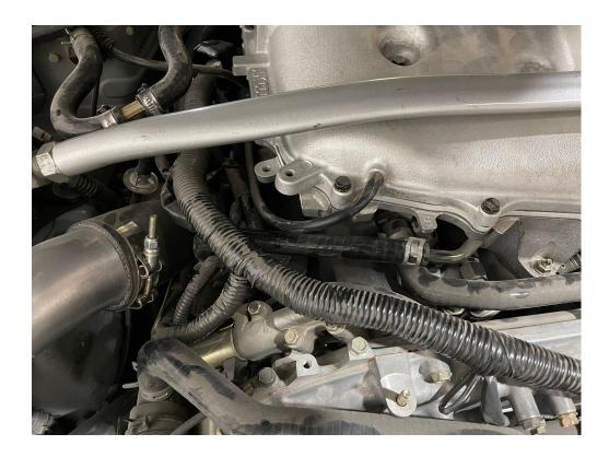
2. Using the smaller 12mm silicone cap, block off the open port on the plenum that the PCV hose was just removed from. Secure with the stock clamp
